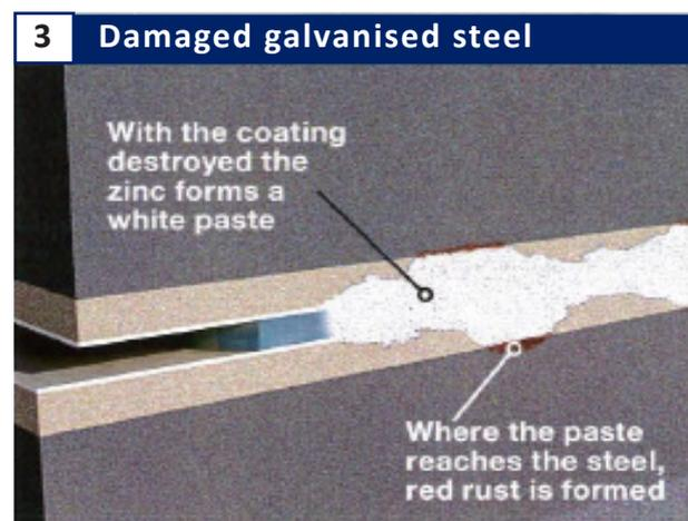
A stack of such surfaces can have the zinc coating destroyed rapidly. This 'white rust', will be found between any two galvanised surfaces stacked wet and touching. As soon as enough zinc has been used up, red rust will start. If the water between the surfaces is saline the corrosion will be greatly accelerated.
