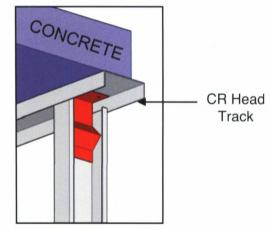
\* CR Head Track required for 100,150 deep studs @ 1.2 gauge and 1.5 gauge
